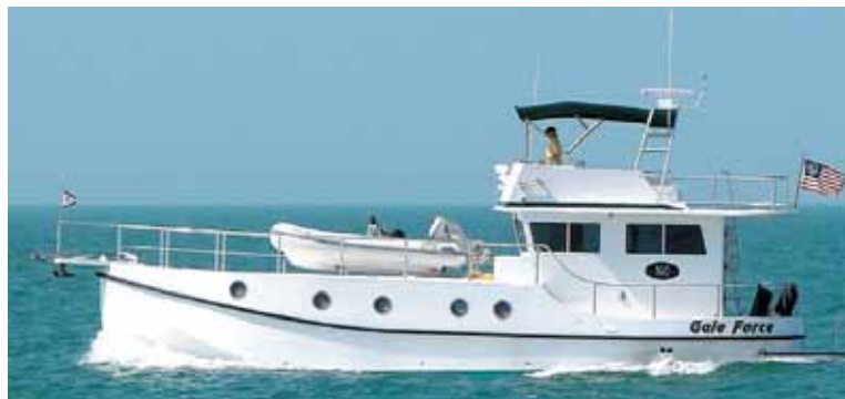
Form stable hulls deliver a comfortable ride without having to rely on finicky, expensive stabilizer systems.
