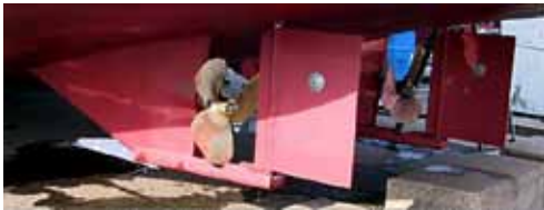
All Great Harbour Trawlers feature twin keels and protected running gear
