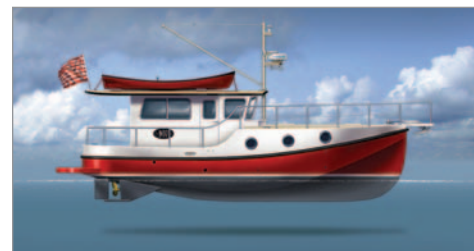
The hull of our N37 shares the same characteristics of all Great Harbour hull designs: shallow draft, wide beam and low center of gravity resulting in a highly stable ride. Twin keels not only protect the props, but make it possible to “careen” the boat during low tide for bottom cleaning and maintenance.
